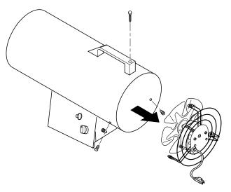
Figure 10 - Removing Motor and Fan Guard from Heater
